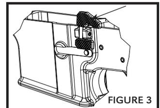
6. Perform function test by manipulating the bolt catch. The bolt catch should rotate freely without the presence of binding or grittiness.
