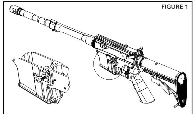
3. Temporarily hold the bolt catch in place using a punch.
